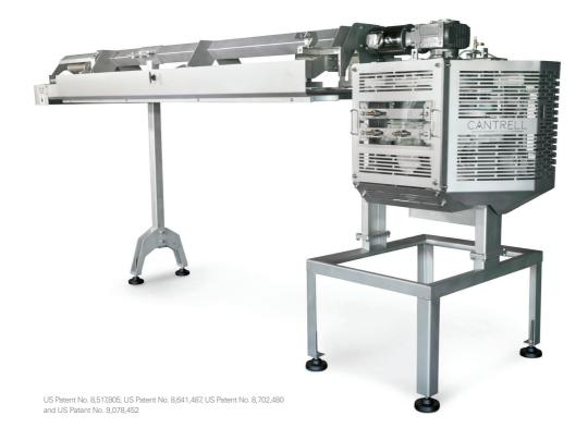
The Cantrell Wing Segmenter offers flexibility, accuracy and ease of use to your operation. The machine is capable of processing up to 180 wings per minute on a processing line or as a standalone application. The Wing Segmenter properly orients the wing at any line speed for accuracy on each individual cut.
