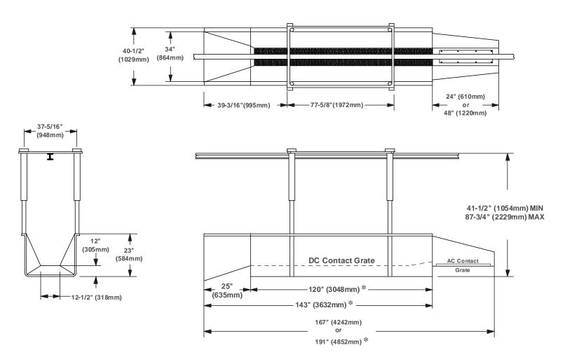
(\*) By special order, stunner length may be extended by adding 24"(610mm), 48"(1220mm), or 72"(1830mm) sections. Dimensioned from the top of the conveyor line to the contact grate with the cabinet "down". The cabinet is manually adjustable "up" approximately 17 1/2 inches.
